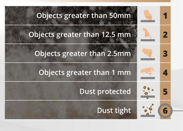
IP, standing for an Ingress Protection is often found in the form of a table. An IP rating is a measure of an enclosure or cases ability to resist items entering it.
